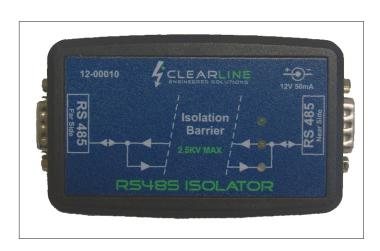
The RS485 Isolator provides high isolation and surge protection for any RS485 bus carrying data signals from a host computer to peripheral devices. Applications include access control and monitoring systems. No setup for baud rate is required as the device is transparent to dataflow. The unit is powered from a mains adaptor and draws 50mA at 12VDC. Indicators have been provided for power, RX and TX data.
